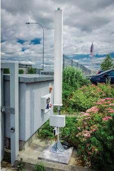
**NuClearance-Med Lite** - **cost effective** portal monitoring system providing essential monitoring to detect radioactive material accidentally disposed of in nonradioactive waste routes.
