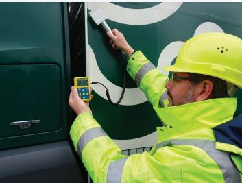
**NuSEARCH Kit** - A choice of detectors designed to easily search for the contaminated material and provide essential information to the nuclear authorities. The combination of the easy-to-use handheld device DolMo and ahighly sensitive probe allows the user to **confirm the presence of radioactivity and trigger the adequate response.**
