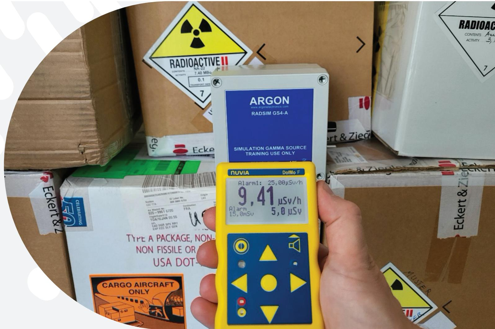
The new training devices DoIMo SIM (dose and dose rate meter) and CoMo-170 SIM (contamination detection device) are designed for the practice-oriented training of radiation protection officers and first responders. The technically modified devices respond to radio waves (DoIMo SIM) or to magnetic fields (CoMo SIM) and can therefore be used for training scenarios even without radioactive sources.
