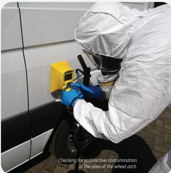
Checking for radioactive contamination in the area of the wheel arch.
