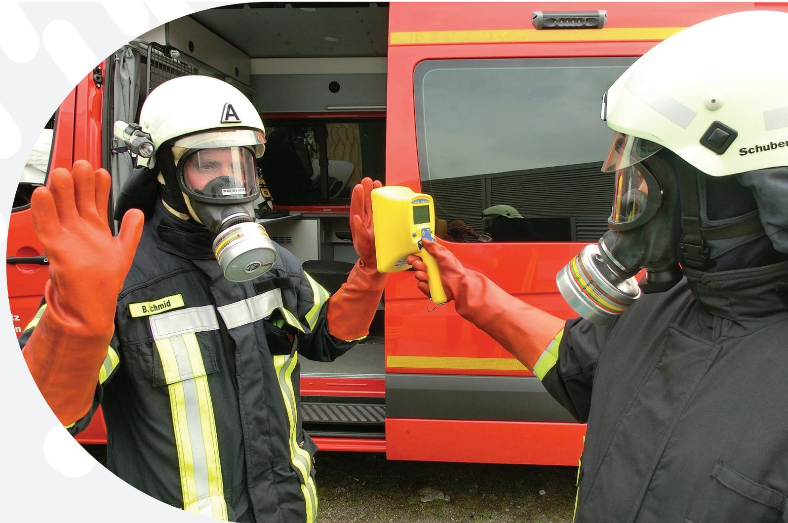
The new training devices DoIMo SIM (dose and dose rate meter) and CoMo-170 SIM (contamination detection instrument) make the practice-oriented training of radiation protection officers and first responders possible. The technically modified devices respond to radio waves (DoIMo SIM) or to magnetic fields (CoMo SIM) and can therefore also be used for training scenarios without radioactive sources.
