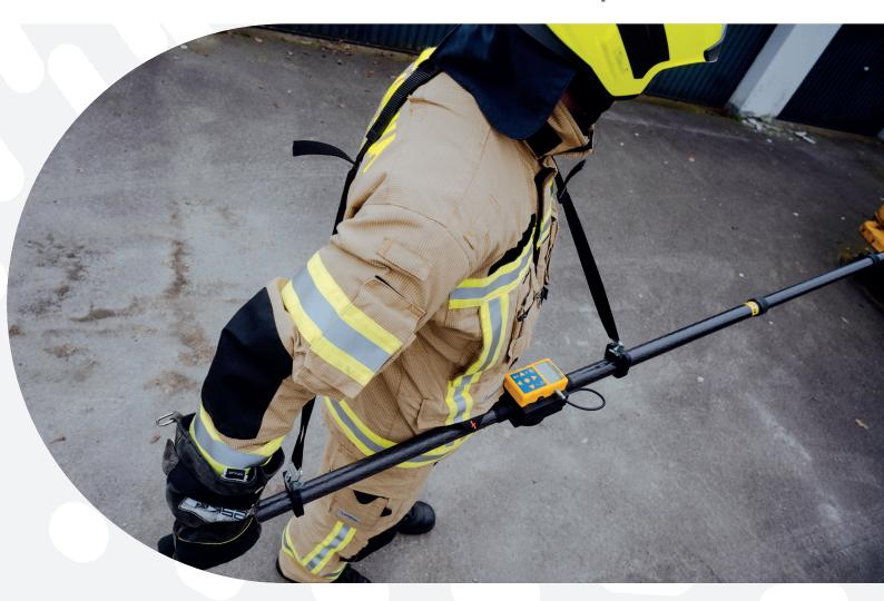
Our new DolMo-Telescope expands our DolMo product line as well as the versatile NUVIATech probe range. It enables precise measurements from a safe distance.
